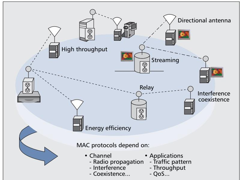
■ **Figure 5.** MAC protocol issues of 60 GHz WPANs: high throughput, directional antennas, relay channels, video streaming, and interference and coexistence.
