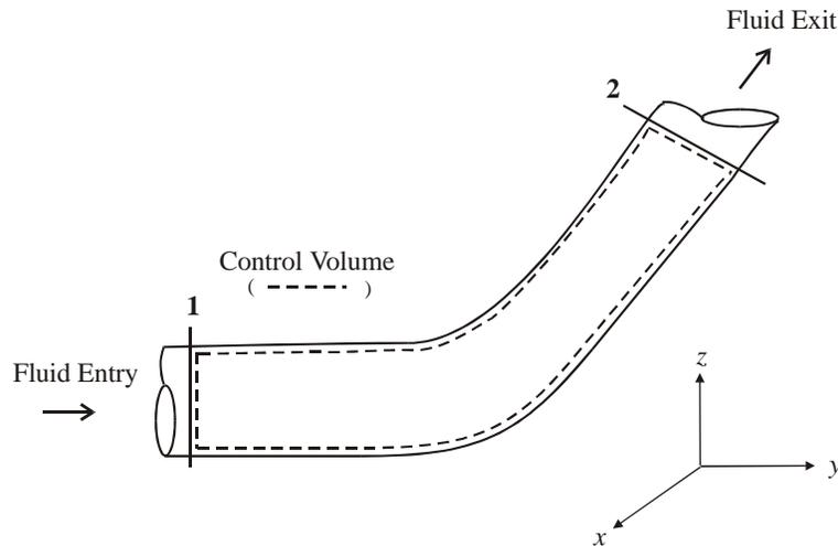
$$0 = \iint_{A_1} \rho v_x v_1 dA - \iint_{A_2} \rho v_x v_2 dA + \iiint_{V'} B_x dV' + \iint_A dF_{sx} \quad (22)$$
